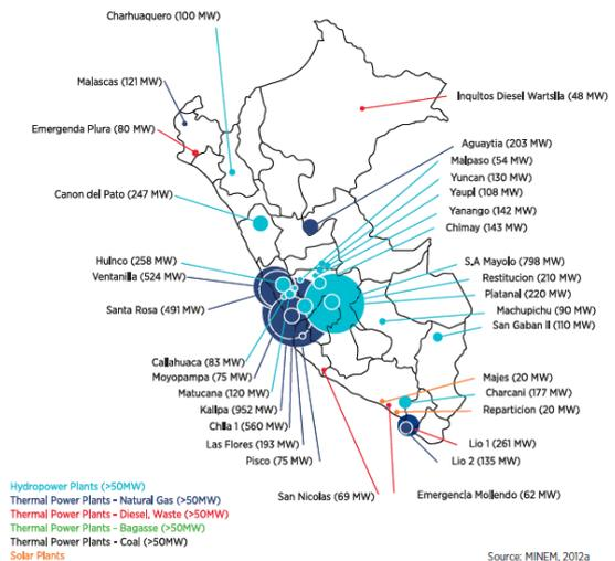
Figure 1. Existing Power Generation Peru by source (MINEM, 2012)
