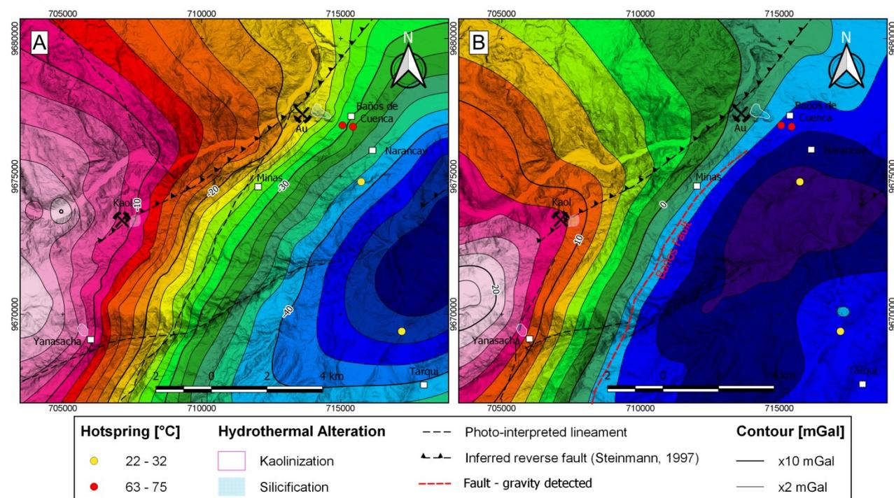
**Figure 4: A. Complete Bouguer Anomaly. B. Complete Bouguer Anomaly without topographic distortion. Note the detected Baños fault.**
