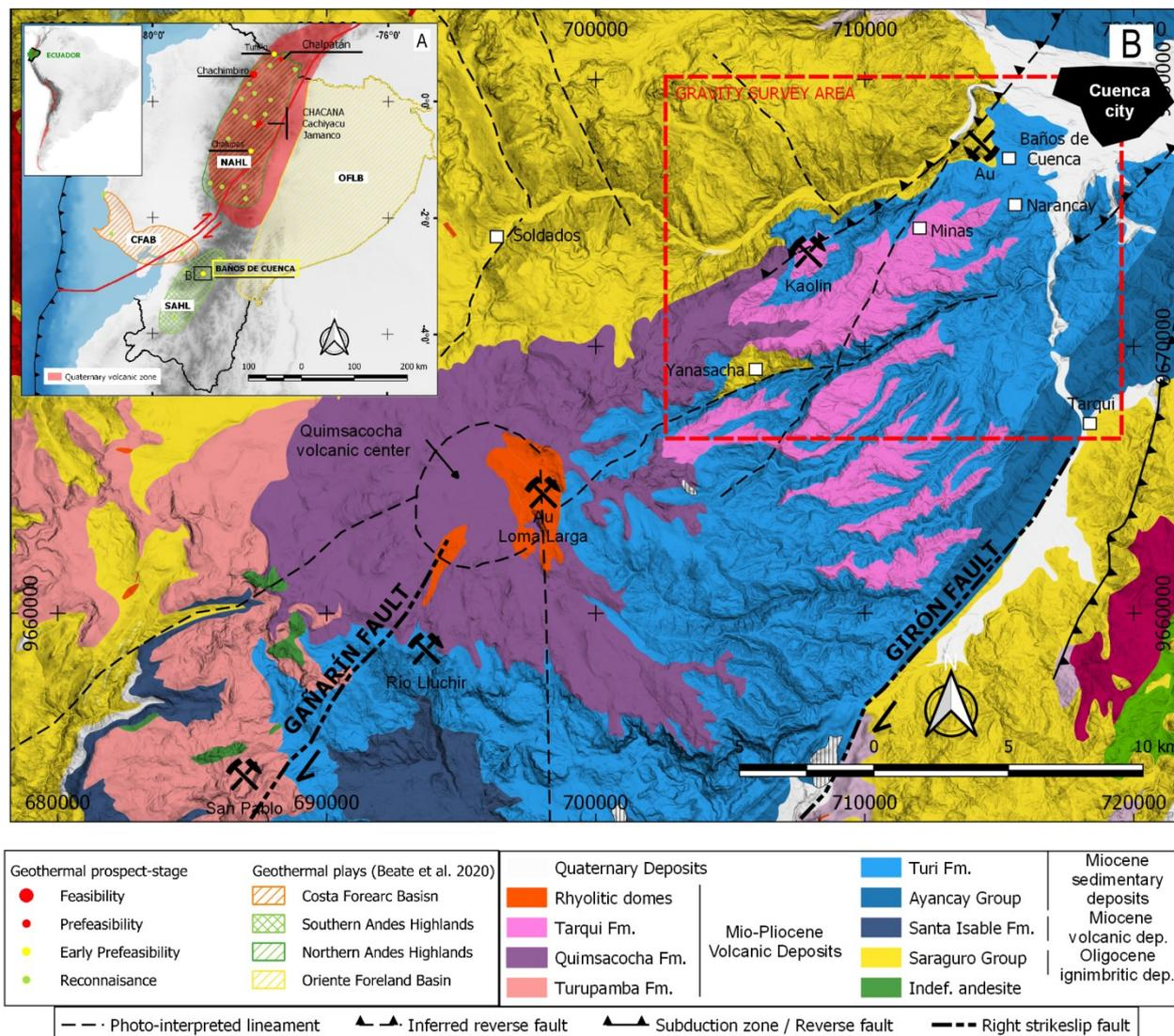
**Figure 1: A. Location of Baños de Cuenca geothermal prospect. B. Simplified geological map with location of gravity survey area. Note the location of mining areas along Gañarín fault.**
