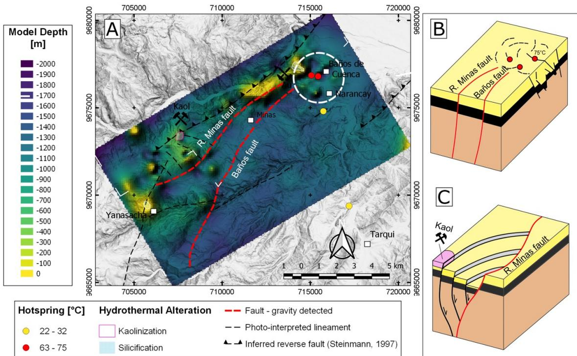
**Figure 6: A. Depth of gravity basement (in meters) with density contrast of 0.5 g/cm<sup>3</sup>. White lines show the direction of section in Figure 7. B. Accommodation structure model for Baños de Cuenca town. C. Extensional duplex structure model-negative flower termination, for southeastern part of R. Minas fault (Modified from Woodcock & Fischer, 1986).**
