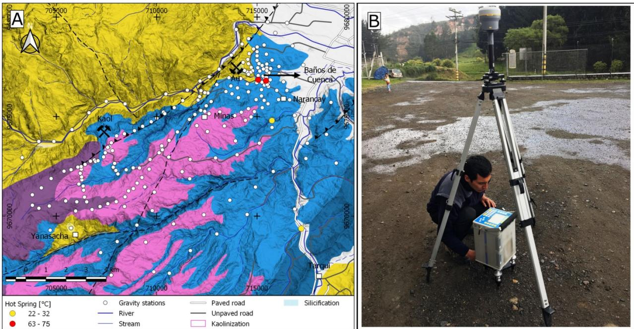
**Figure 2: A. Simplified geological map of gravity survey area with the location of gravity stations. Additional symbols please refer to Figure 1. B. Instrumentation for the field survey.**
