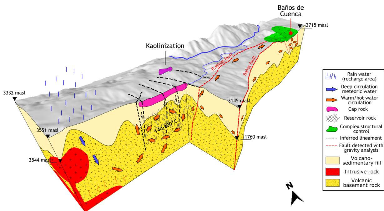
**Figure 7: Preliminary model for Baños de Cuenca Geothermal prospect. Depth of volcanic basement (Saraguro group) was extracted from 3D gravity inversion.**
