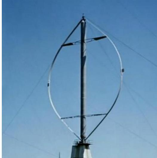
**Figura 4 Aerogenerador Darrieus (Fuente: Boston University, Mechanical Engineering)**
